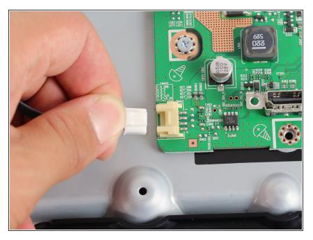
Disconnect the navigation button from the motherboard by holding down the thumb tab and pulling its connector out.
