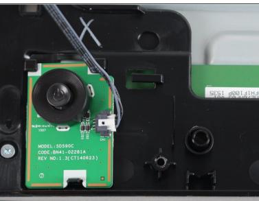
Remove the navigation buttons connector wire from the monitors body tab.
