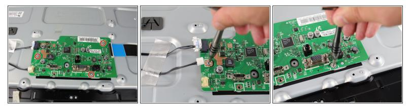
Remove each of the 5mm length screws attaching the motherboard to the body of the monitor using a #1 Phillips head screwdriver.
