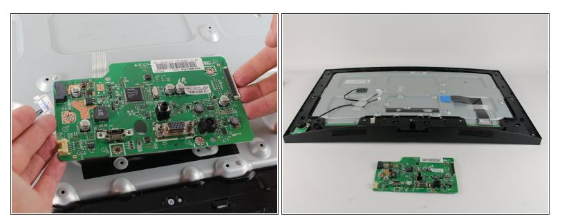
• Using both hands, lift the board off of the monitor body by the motherboards base.
