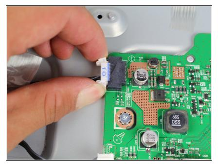
• Remove the screen connector by gripping its sides and gently pulling while wiggling back and forth.
