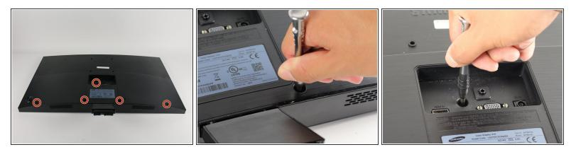
• Use the #1 Phillips head screw driver to remove each 13.75mm length screw from the rear panel.
