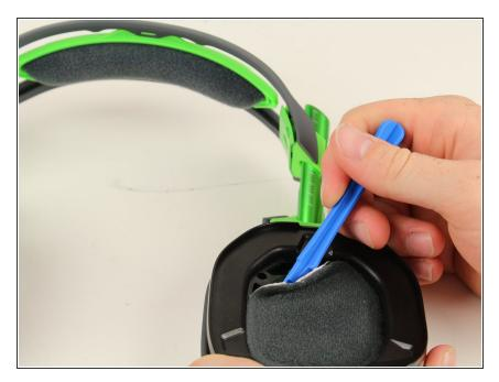
Squeeze the plastic opening tool between the black plastic and foam pad on non mic side and then pry upwards to remove the felt pads covering the speaker.
