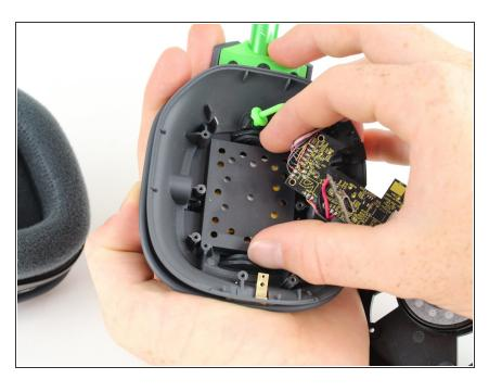
Remove the back panel by squeezing the two tabs together and pushing out.
