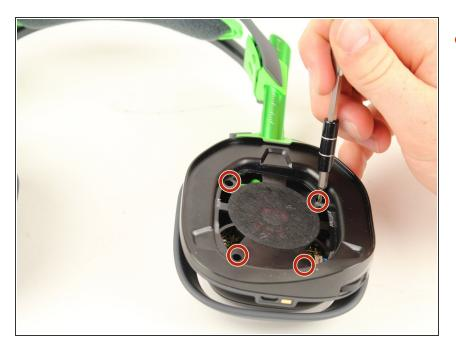
Remove the four 6mm Phillips 1 screws.
