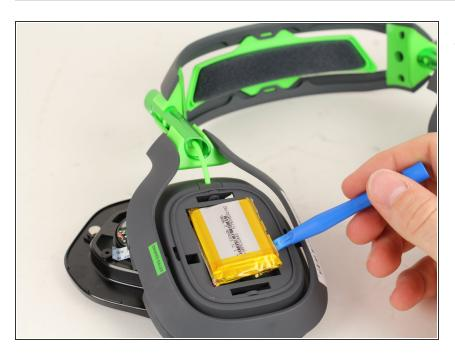
Remove the battery by using the plastic opening tool to pry it away from the headset.
