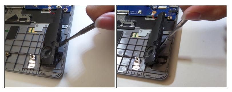
• Remove the speaker by lifting it up and away from the laptop.
