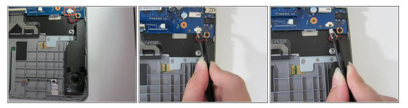
• Using the fine tipped tweezers, detach the white power clips from the motherboard.
