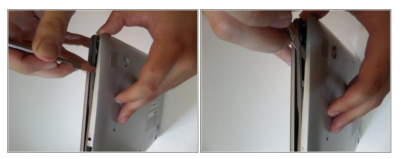
• After deconnecting all the brackets, pull the back panel away from the laptop.
