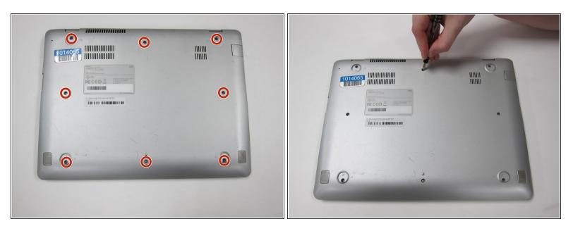
• Remove the eight 7mm screws using the J0 Screwdriver.
