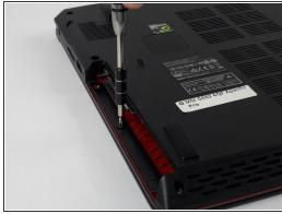
• Remove the three PH #0 2mm screws that were hidden underneath the optical drive.
