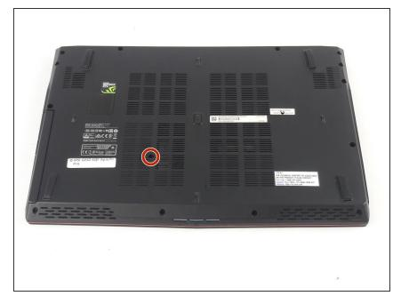
Use a Phillips screwdriver to remove the 5mm screw securing the optical drive to the bottom case.
