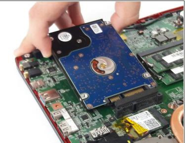
Remove the hard drive by gently lifting up and pulling the drive out of the connection slot
