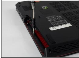
Remove the three PH #0 2mm screws that were hidden underneath the optical drive.
