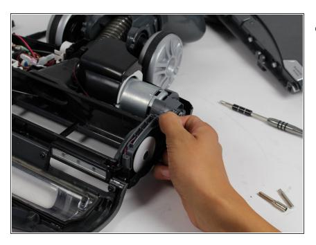
Remove the black belt located on the right face of the vacuum nozzle.
