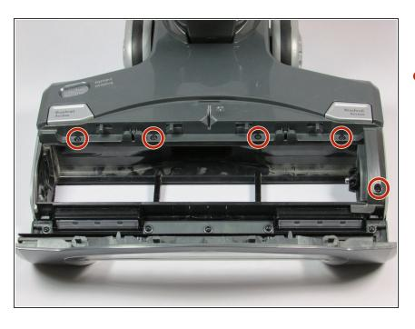
Remove the five 5mm Torx #9 screws on the front side.
