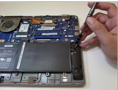
Remove the four 3mm screws holding the battery with the J0 screwdriver.
