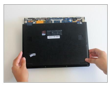
Now that the screws are removed, gently lift the back panel upwards to detach it from the rest of your laptop.
