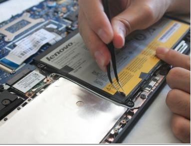
There may be tape around the edge of the battery to secure some wires. Use a pair of tweezers to remove the tape so that the wires are no longer attached to the battery.
