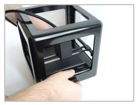
Removing the frame is necessary to access the z axis belt, motors and ports. Make sure the unit is unplugged and set on a hard level surface.
