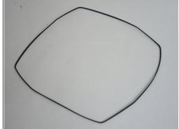
Remove the z axis belt from the device by simply lifting each corner of the belt off the corner gears and slide up over the z axis bars.
