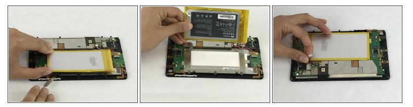
• Use the plastic spudger to remove the battery from the device that is glued on the metal frame.
