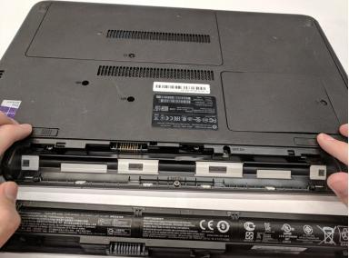
Once the releases are in position, pull the battery out.
