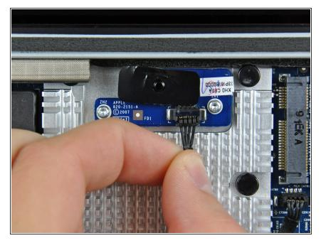
Disconnect the IR sensor cable from the IR board by pulling its connector toward the bottom edge of your iMac.
