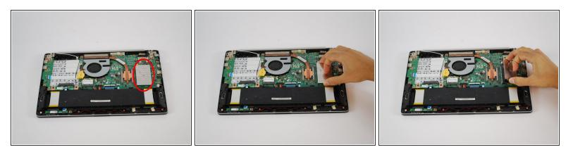
• Remove the top covering the RAM chips.
