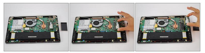
• Remove the RAM from the device.
