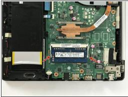
Now the RAM stick is exposed. Using two fingers, gently push the buttons to release the RAM stick
