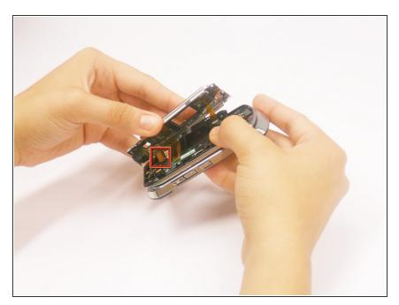
Use the flat end of the plastic opening tool to unclip the cable ribbon from the logic board
