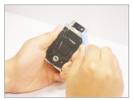
Using the plastic opening tool, peel back the plastic cover that is glued on top of the camera lens.
