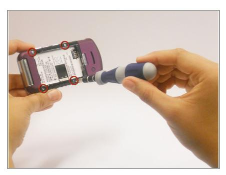
Using the T5 Torx-screwdriver, remove the four 5.5 mm screws on the back panel.
