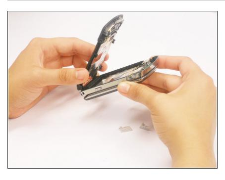
Remove the plastic covering completely from the body of the phone.
