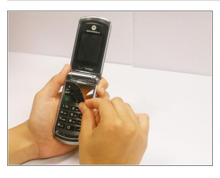
After removing the main logic board, use the plastic opening tool to poke from the back and peel off the key pad cover. To reassemble your device, follow these instructions in reverse order.
