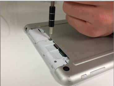
Using the Phillips Head #000, unscrew the 5 4mm and 3mm screws at the top.
