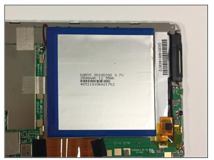
(i) The battery is the large, silver square inside the tablet. It is connected to the motherboard by two wires.
