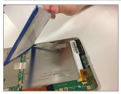
Peel off the battery from the device to completely remove it.
