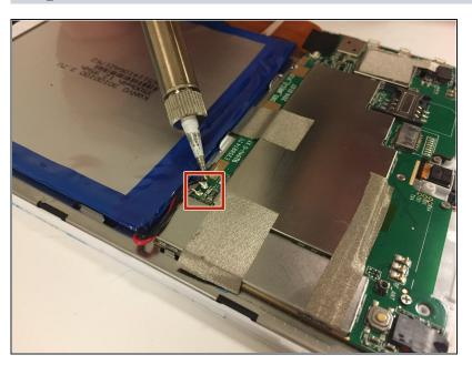
Use the soldering iron to remove the two metal ends that connect the battery to the motherboard.
