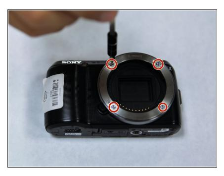
Use a Phillips head 000 screwdriver to remove the four 5.0mm screws on the E-mount.
