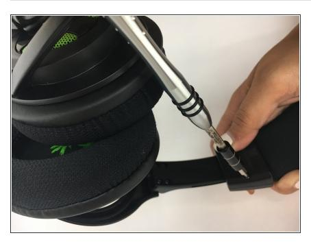
Remove the two 1.10 mm screws using the a T3 screwdriver.
