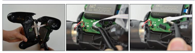
• Pull the ribbon cable out of the motherboard port to fully separate the two halves, using a pair of tweezers.
