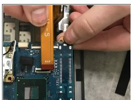
Remove the white and orange cables attached by pulling out the cables
