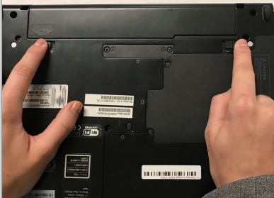
Unlock the clips by pulling towards the unlock.
