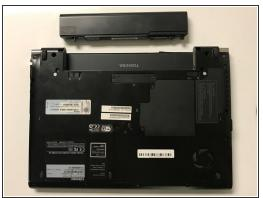
Holding the unlock clips push the battery away from the laptop.
