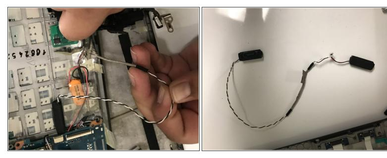
Once the cable had been released you have successfully removed the speakers!
