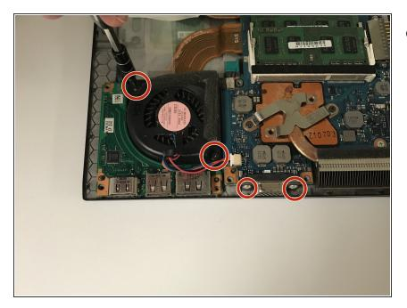
Remove the screws from the fan and side ports
