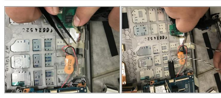
Using the tweezers, gently remove the tape being used to hold down the speaker cables.
